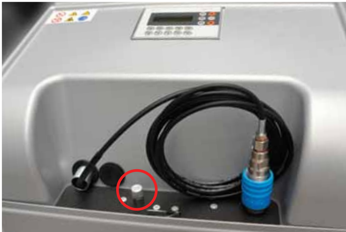
Oil dip stick position on service panel.
