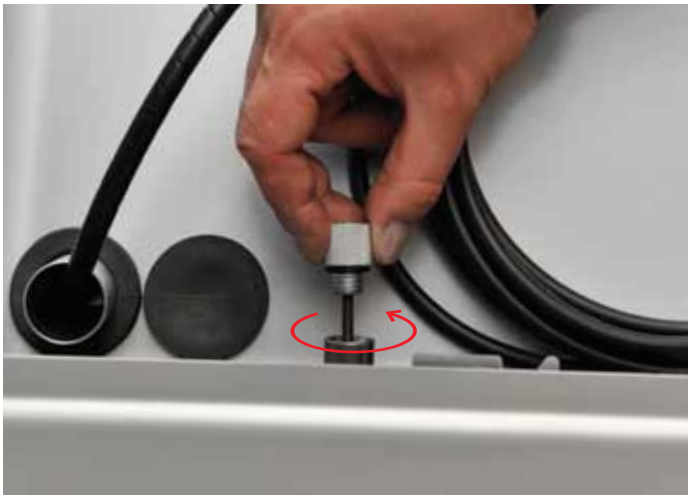
Oil dip stick must be unscrewed during oil check.
